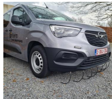
Gas leak detection on buried pipelines by car and on foot
