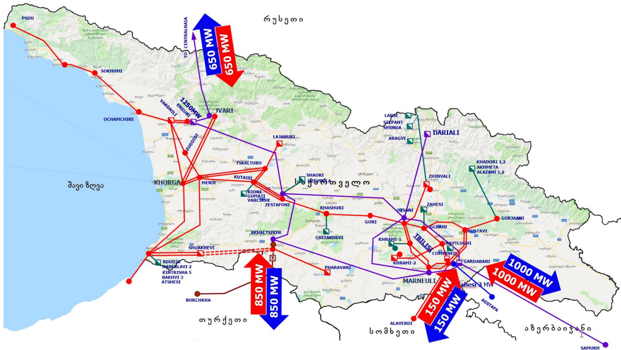
Fig. 7 Cross-border transfer capacities between power systems of Georgia and its neighboring countries
