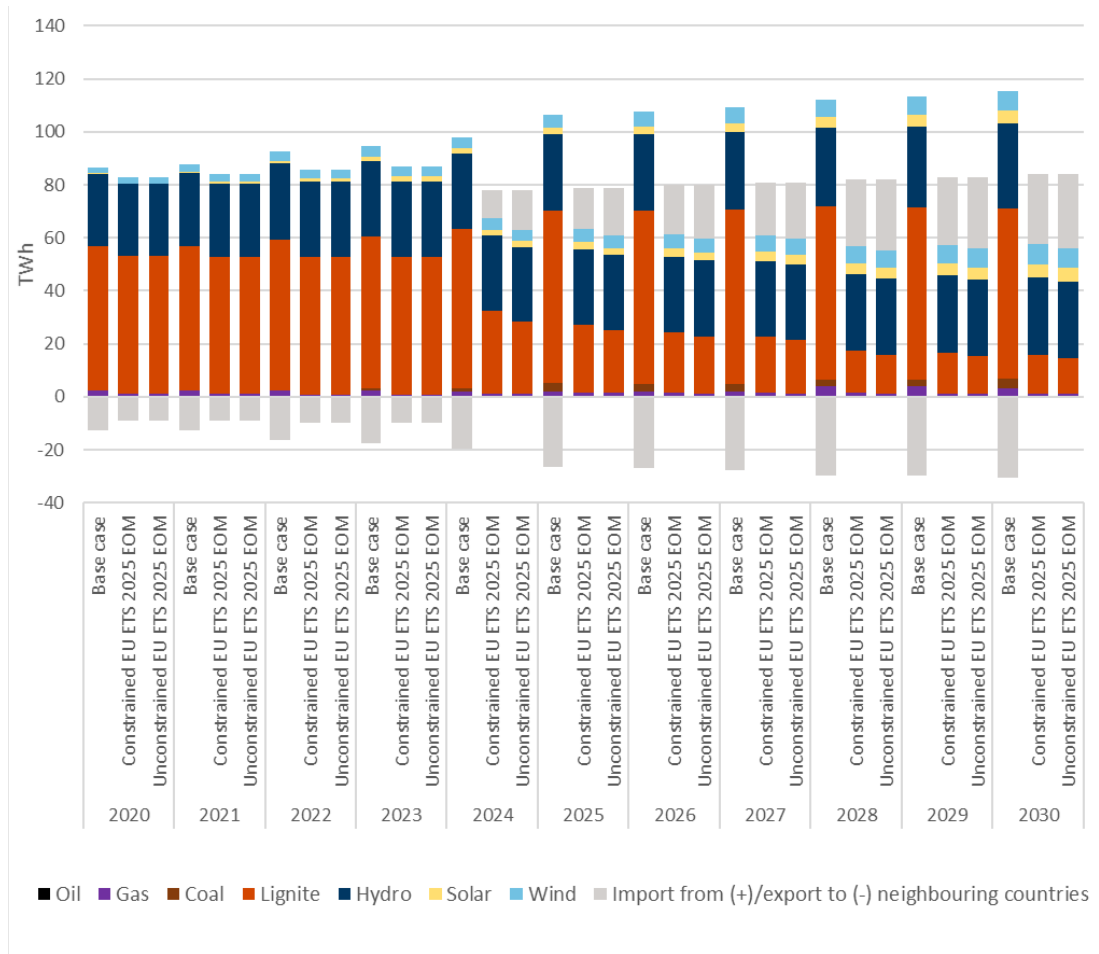
Figure 34: Generation outlook in the WB6 region, per technology in the constrained EU ETS 2025 Energy Only scenario (TWh)
