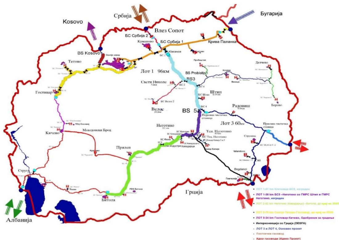
Figure 78. Natural gas transmission system of Macedonia
