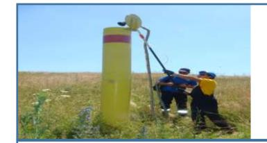
Methane detector is sampler unit Hi Flow Sampler structurally safe tool powered by a built-in battery. It provides the ability to accurately measure the volume and intensity of natural gas leakage from any pipeline fittings and seals at the facilities main gas pipelines.
