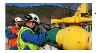
→ 2022 LDAR campaign compatible with regulation project with detection level at 500 ppm
