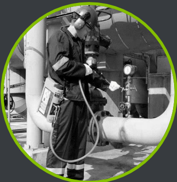
LDAR Fugitive Emission Management HFS / PID / FID
