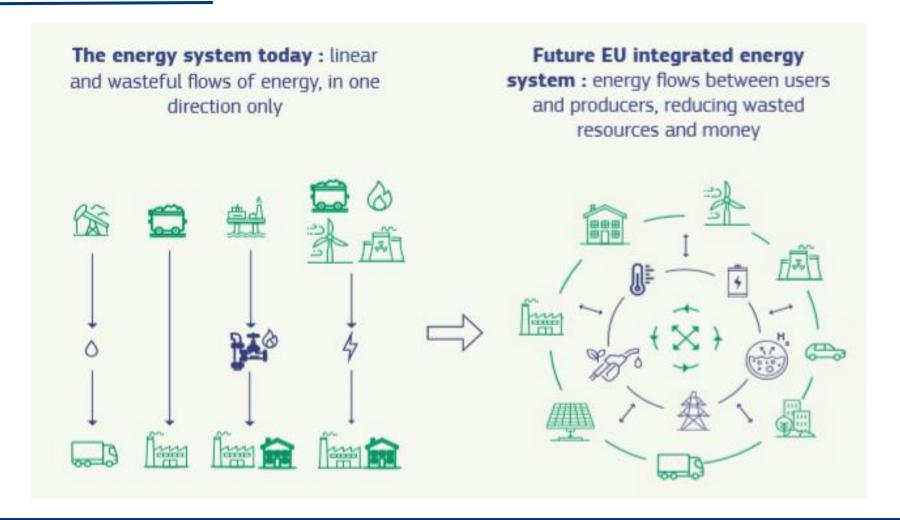
**Energy System Integration (ESI)** is the integrated planning and operation of the energy system 'as a whole', across multiple carriers, infrastructures and consumption sectors
