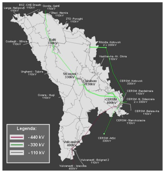
Figure 7. Layout of the HV transmission network of the RoM
