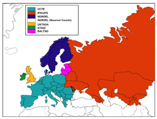
Figure 5. Major synchronous transmission grids in Europe and CIS
