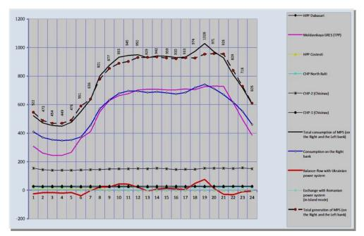
Figure 12. Load diagram and meeting the demand on a day of absolute peak in 2015 (MW)
