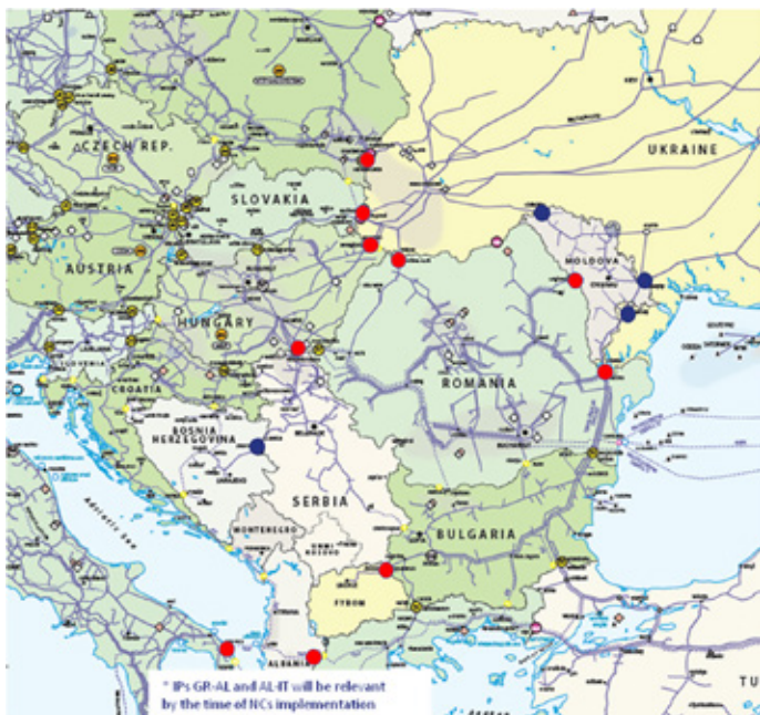
Figure 5 Interconnection points between transmissions networks of Energy Community Contracting Parties and European Union Member States
