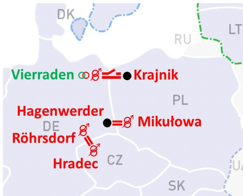
Reconnection of the Krajnik-Vierraden line with PSTs in Vierraden substation plus the nearest PSTs in the region. Transitional state until the completion of the project, referring to PSTs on the PL-DE border.
