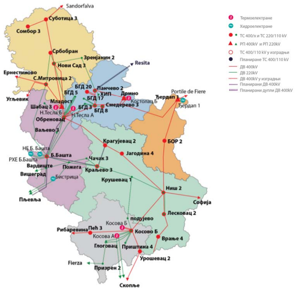
Figure 16: Transmission system of Serbia and Kosovo* (existing situation with planned reinforcements) 11 Source: EMS
