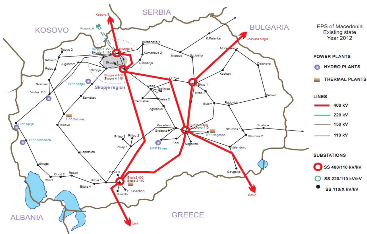
Figure 4. Single-line diagram of Electric Power System of Macedonia, year 2012
