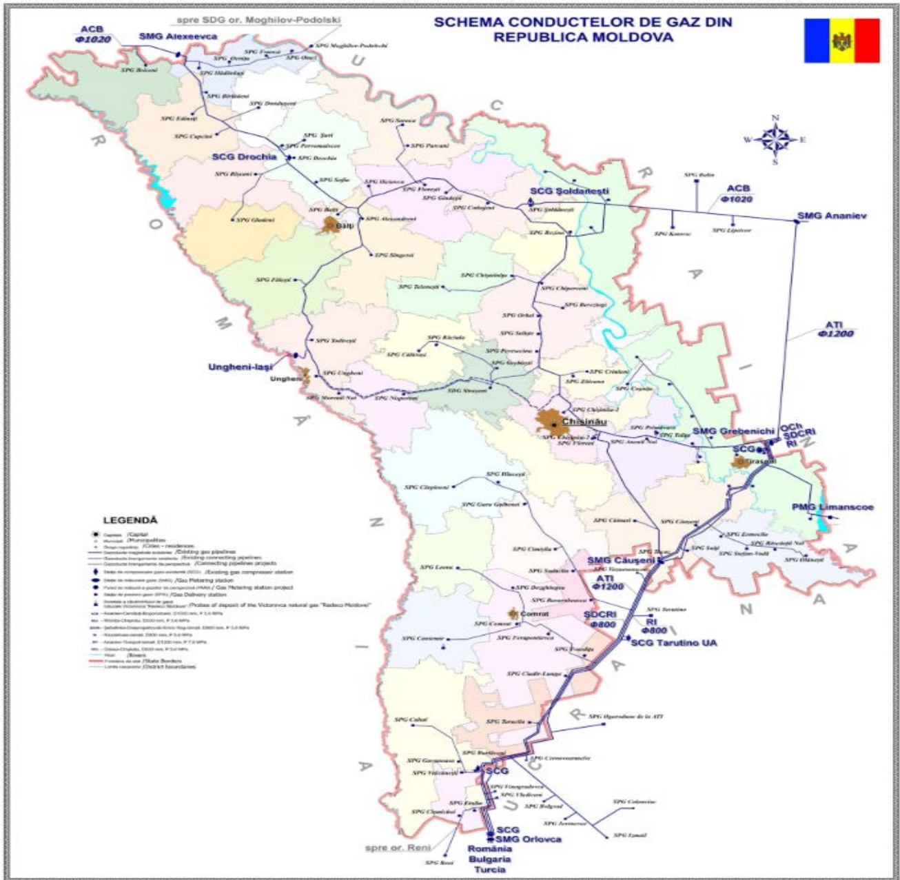
Figure 15. Infrastructure of the natural gas transmission system on the territory of the Republic of Moldova
