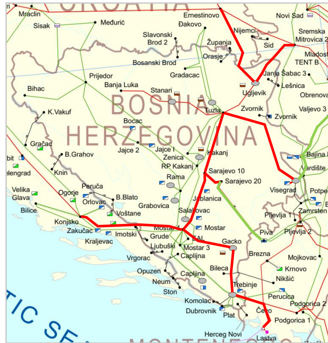
Figure 80 Structural congestion elements in Bosnia and Herzegovina
