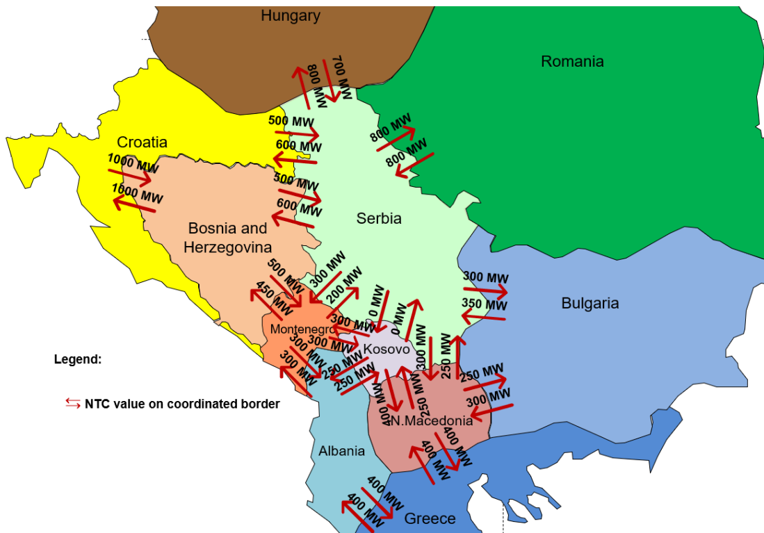
Figure 23 NTC values for the given example graphically represented in the coordination area
