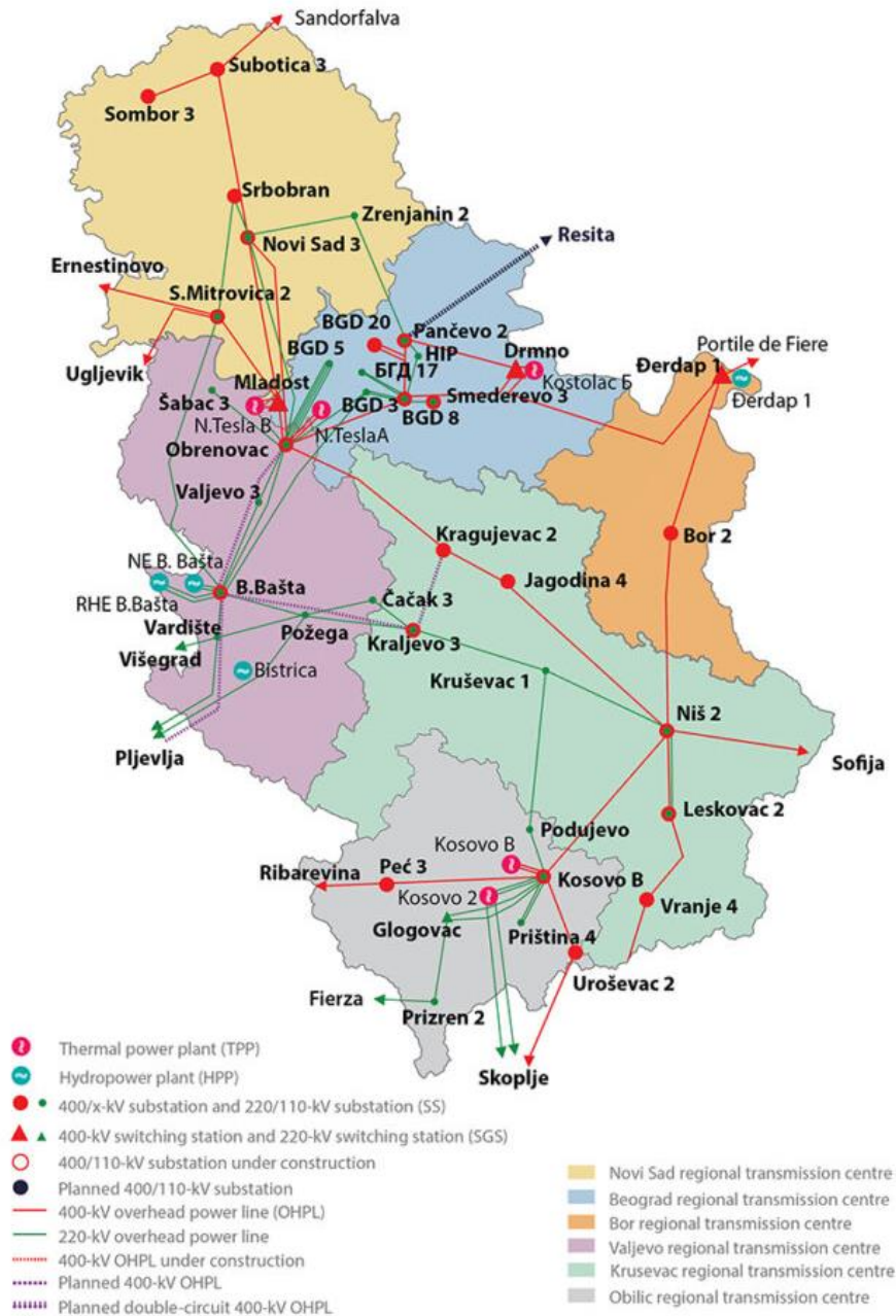
Figure 16 400 and 220 kV transmission network in Serbia (and Kosovo*) in 2022
