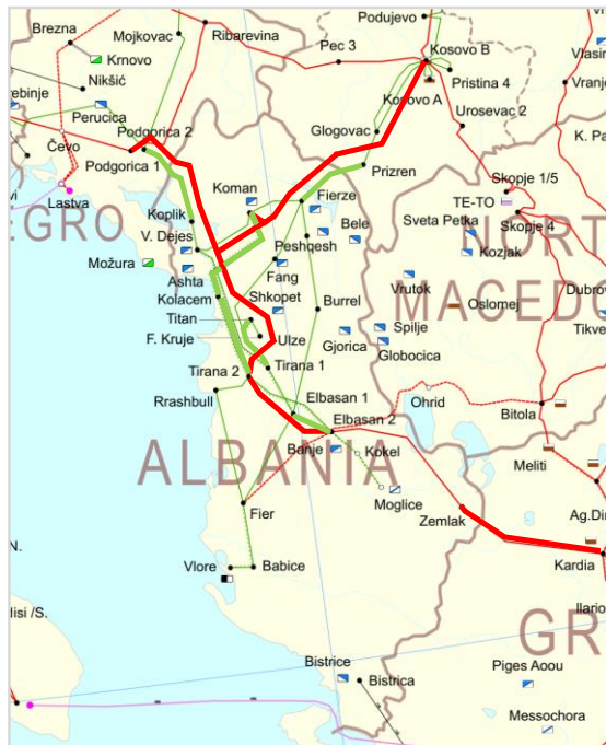
Figure 79 Structural congestion elements in Albania
