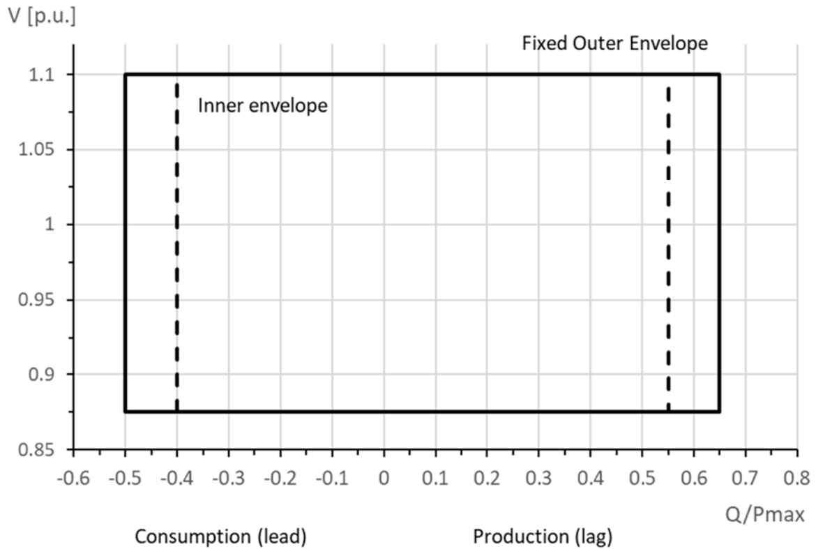
Figure 52 - U-Q/Pmax profile envelopes applicable to type C and D SPGMs
